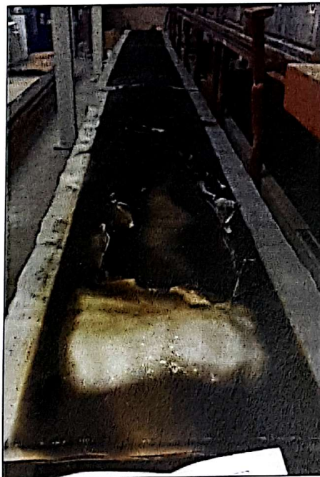
Photo 3: Specimen after the test (located near the fire end)
